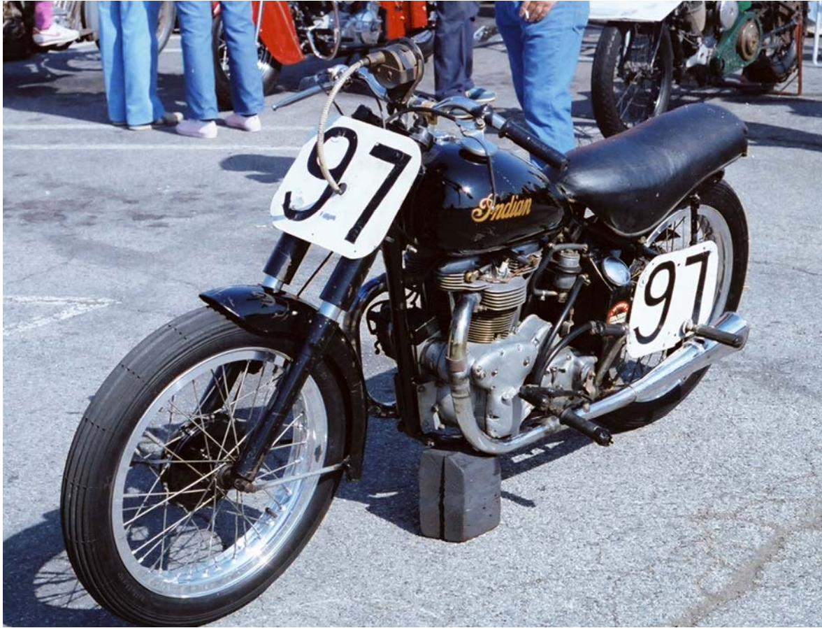
(Fig.8) Looking at the Murdaugh Warrior from a left front \frac{3}{4} view you can clearly see the adapter for the Edison-Splitdorf RM magneto. The remote float bowl is in view as well. The use of 19" Boranni rims is an advantage for this bike, which appears to be set up for Laconia with its sharp left and right-hand turns, allowing the motorcycle additional ground clearance. This machine is a treasure in that it allows us an unmolested glimpse into the world of racing motorcycle preparation as it truly appeared in days gone by.
