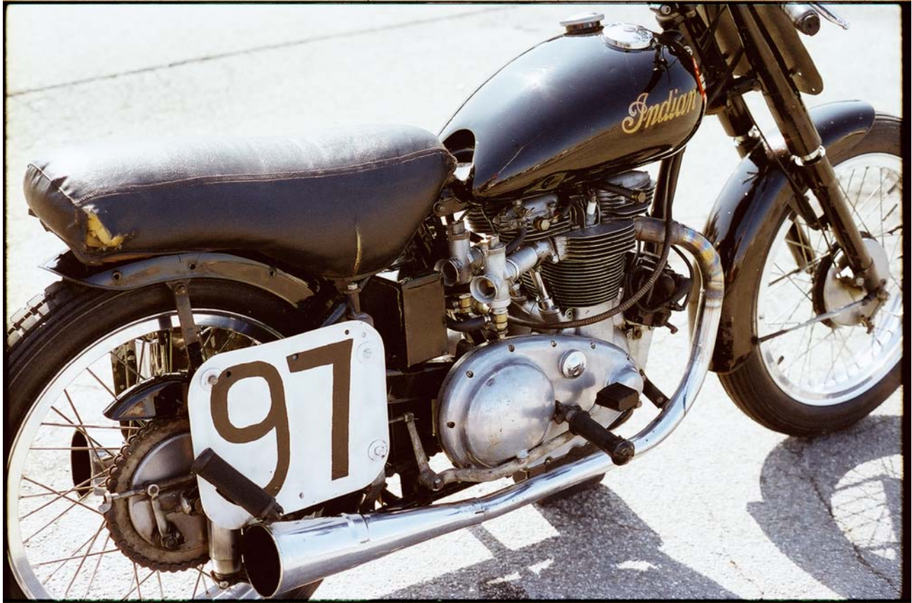
(Fig.7) This right side view of Clem Murdaugh's racing Warrior clearly shows the application of dual Amal 276 carburetors and the Edison-Splitdorf RM model four cylinder type magneto. Notice the simple fabricated appearance of the intake manifold. Also visible in this view is the megaphone exhaust. One can only imagine the sound at 7,000 RPM. Although appearing homemade, this seat arrangement was a nod towards a more modern European style of road racing making it more comfortable for the rider and easier for him to slide back and forth on the seat as the bike was entering or exiting a turn.
