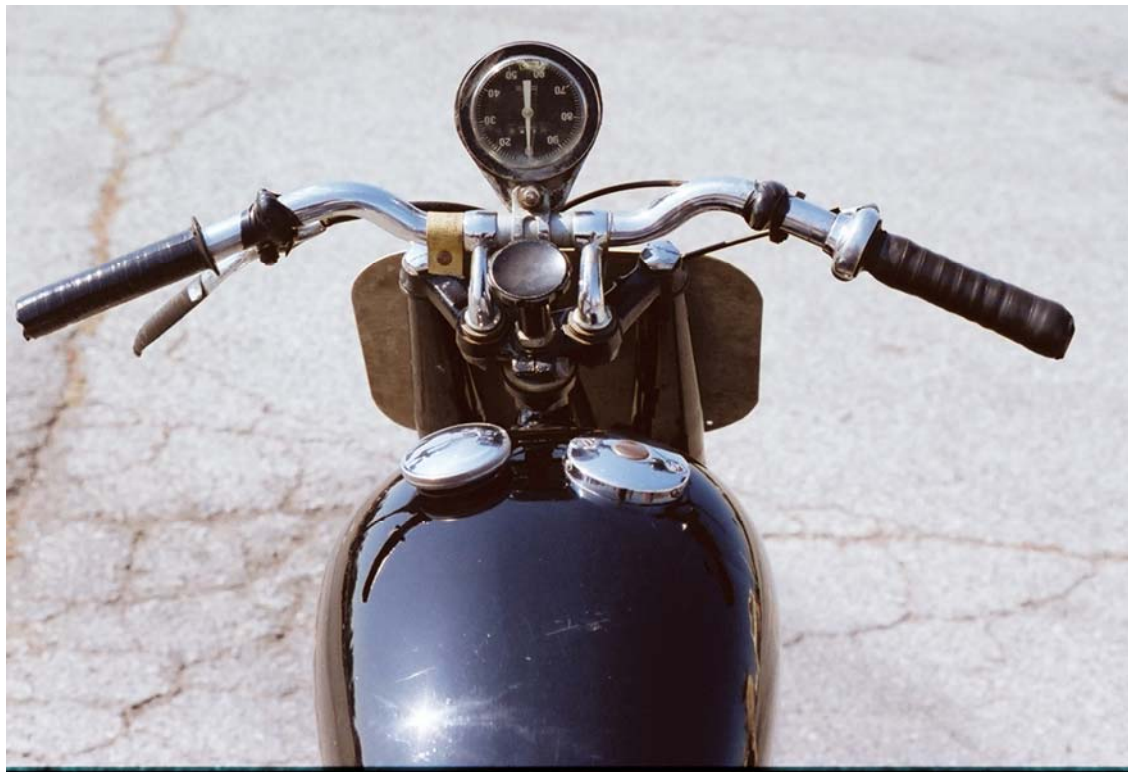
(Fig.9) Here is the view that Clem Murdaugh and Dave Henry experienced while riding the Warrior at high speed on the racetrack. Notice that the tachometer dial is in an inverted position. This was done so that the redline would be at the 12 o'clock position for easy reference by the rider while involved in the race. The little beige colored strap to the left of the left handlebar riser is the original rider entry tag for the last race this bike was involved in at Laconia. The handlebars, while from the period, represent a nod toward a more modern style of road racing.
