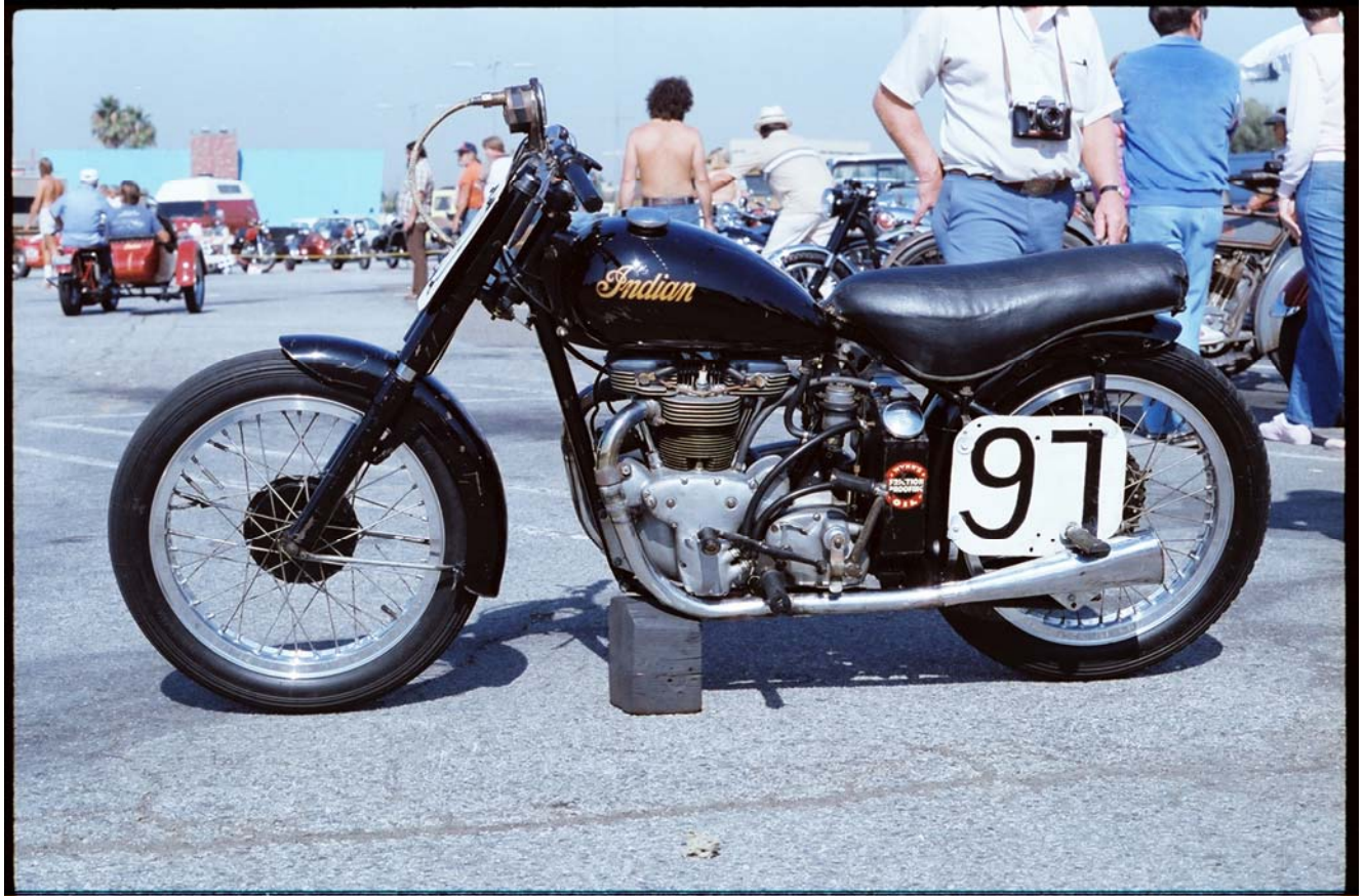
(Fig.6) This pristine unrestored machine, at one time belonging to Clem Murdaugh, represents the Indian vertical twin racing motorcycle in its final most advanced form. From this side the machine presents a pretty typical appearance with a number of the factory accessories being represented including the under seat oil tank, fuel tank with left side petcock, and remote float bowl. What is out of the ordinary obviously is the handlebar mounted tachometer. The real surprises lie on the opposite side however.
