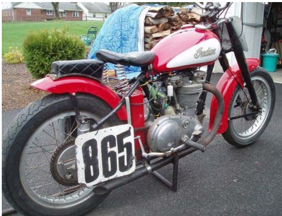
(Fig.5) Here is one of Herb Reiber's Laconia Scouts in current vintage racing trim. This example is great for displaying three of the most notable factory racing accessories associated with the vertical twin racers. These include the factory under seat oil tank, large capacity Daytona fuel tank, and the sand cast 12 fin cylinders. Notice that the fuel tank has two gas caps as opposed to one gas cap and a recess in the tank for the ignition switch and the absence of a notch for the nose of the saddle.
